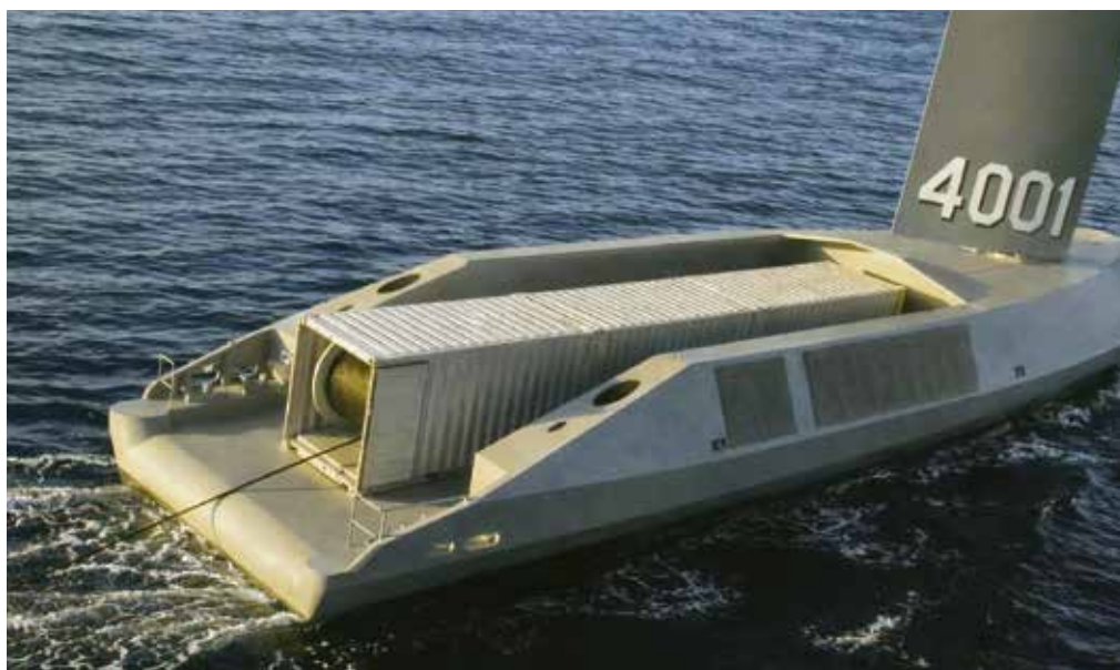
Concept of the Sairdrone Spectre Silent Endurance variant. The 52 metre long stealth-USV can deploy a towed sonar array. Sairdrone is partnering with Fincantieri for construction. (© Sairdrone)
