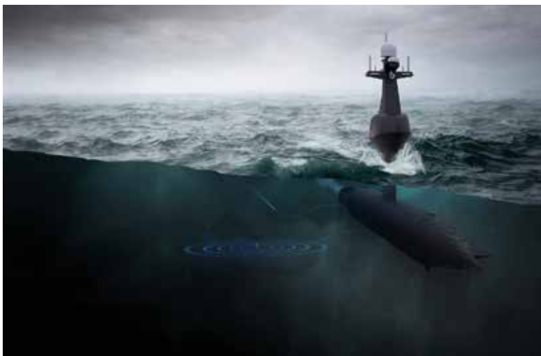
MEKO® S-X SWASH-type LUSV deploying active and passive towed sonar. © TKMS
