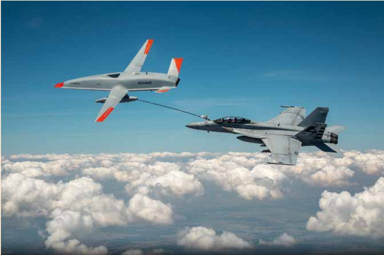
Both the US Navy and the British Royal Navy envision hybrid air wings aboard aircraft carriers. Here the Boeing-developed MQ-25 refuels a US Navy F/A-18 during testing. (© US Navy)
