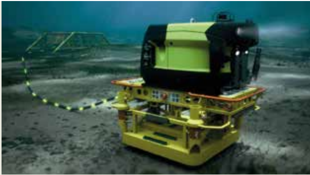
Unplugged uses inductive wireless power transfer: a receiver inside the UUV communicates with a charging pad on a fixed or towed station (© Unplugged)
