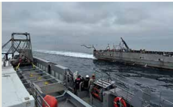
In a test as part of the NOMARS programme, the USV Mariner (right) deploys a refueling probe towards the USV Ranger (left) in the first test of fueling at sea (FAS) without any human interaction required on the part of the receiving vessel. The personnel aboard the Ranger are observers only (© DARPA)
