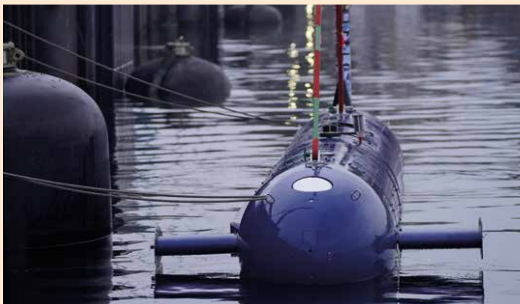
TKMS and IAI delivered the first BlueWhale large autonomous underwater vehicle to the German Navy in February 2026. The autonomous UUV combines reconnaissance, ASW sensor technology and data fusion in a single system. (© Bundeswehr/M. Krönke)
