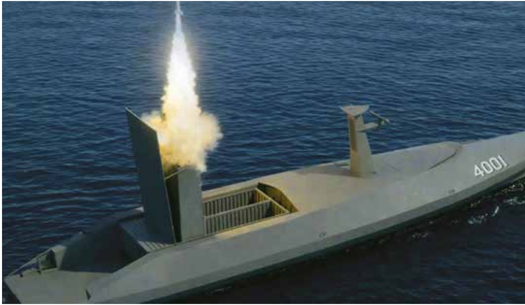
The Spectre Stealth Strike accommodates the Mk 70 Payload Delivery System and achieves a sprint speed of 30 knots. There are currently no orders for the system, but Fincantieri is planning live fire demonstrations during RIMPAC 2027. (© Saildrone)
