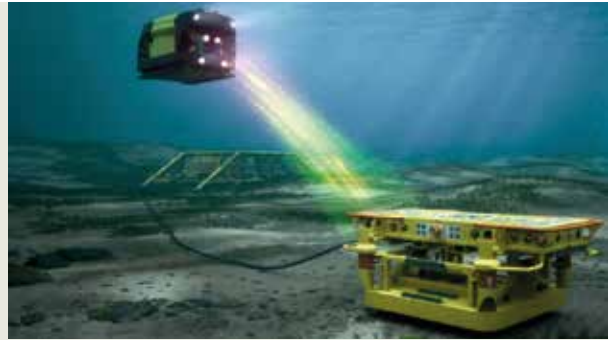
Getting a UUV to within five to ten metres of a subsea charging station is a solved problem; guiding it to docking precision without GPS remains a challenge (© Unplugged)
